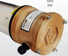
ZNP.X SERIES type fluorescent lamp comprises a lamp tube assemblwith two end caps. The housing consists of a transparent polycarbonateube with polycarbonate end caps. The electronics are located in the main body. Both end caps connected together by two 6 mm diameter tie bars, therefore compressing the tube and caps. The equipment is intended for fixed installation. The equipment has normal fluorescent lamp, led fluorescent lamp and emergency kit variations.
